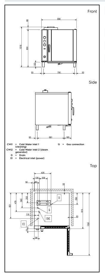
Electric Supply voltage: 220-230 V/1 ph/50 Hz 0.35 kW **Auxiliary**: Electrical power max.: 0.35 kW Gas Gas Power: 18.5 kW Capacity:
